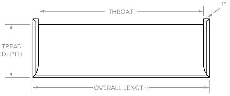
\*OVERALL LENGTH SHOULD BE 2" LONGER THAN THE THROAT TO ACCOUNT FOR RETURN END THICKNESS
